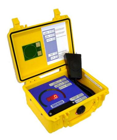
A new state of the art meter capable of measuring the moisture content of various substrates using both pad and pin sensors.
